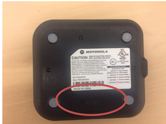
Figure 2 - Date code location in Single Unit Charger RLN6505A (engraved)
