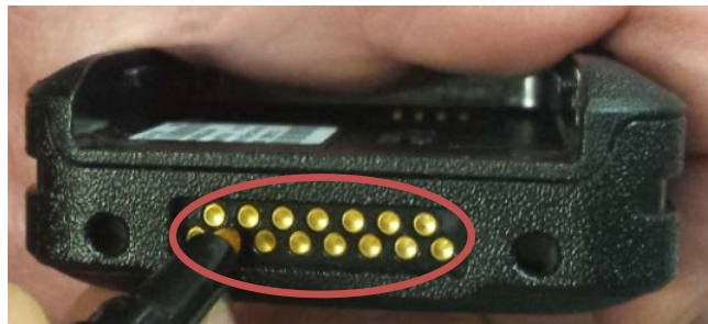
Figure 1 - Minitor VI with I/O connector concave pins
