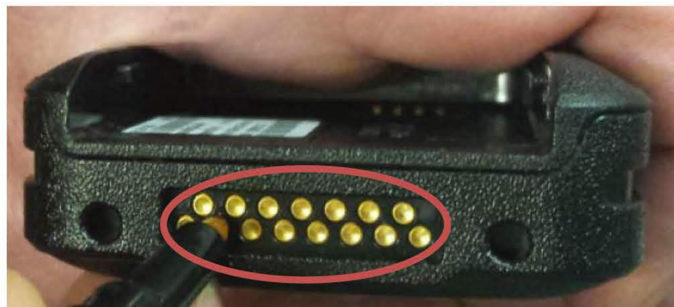
Figure 1 - Minitor VI with I/O connector concave pins
